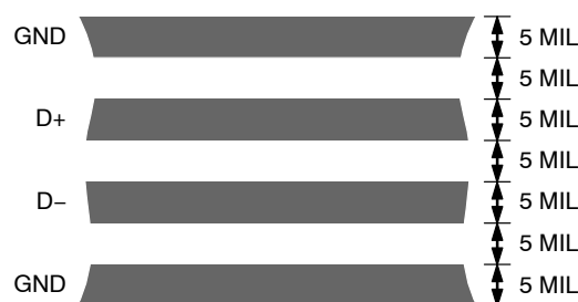
Figure 23. Typical Arrangement of Signal Tracks
