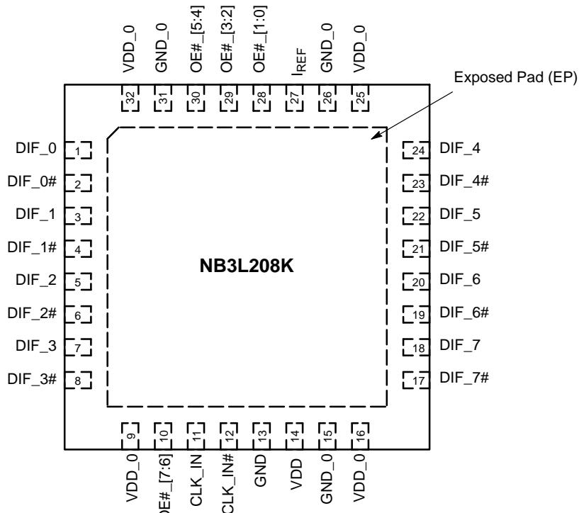
**Figure 2. 32-Pin QFN Pinout**
