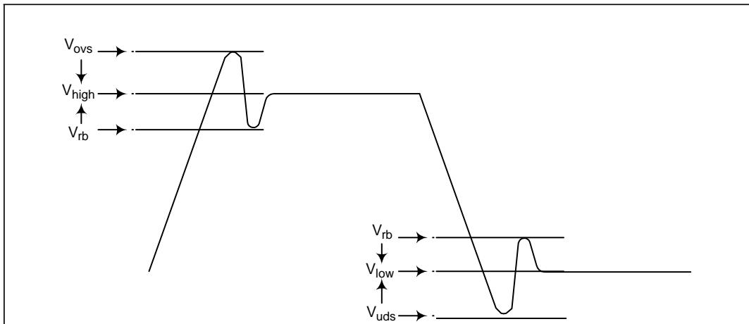
**Figure 14. Single-Ended Measurement Points for V<sub>ovs</sub>, V<sub>uds</sub>, V<sub>rb</sub>**
