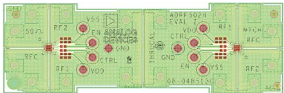
Figure 16. Evaluation Board Layout
