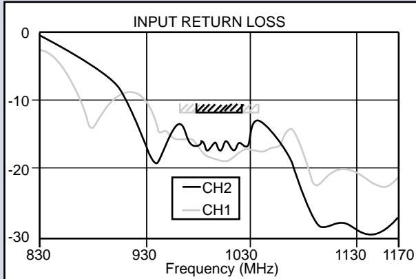
Channel 1 and Channel 2 Input Return Loss Response
