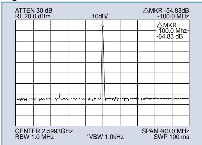
Multiplier Spectral Purity (Close Spectrum @ +85°C)
