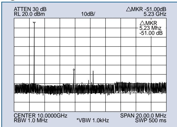
Multiplier Spectral Purity (Wide Spectrum @ 25°C)
