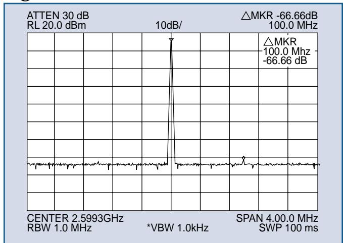
Multiplier Spectral Purity (Close Spectrum @ -40°C)
