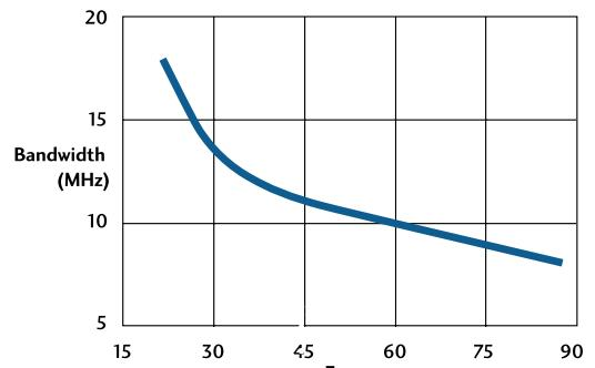
10 dB return loss bandwidth vs. dielectric constant (f = 1575 MHz).
