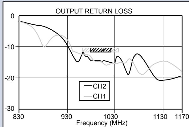
Channel 1 and Channel 2 Output Return Loss Response
