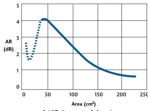
Axial Ratio vs. ground plane size
