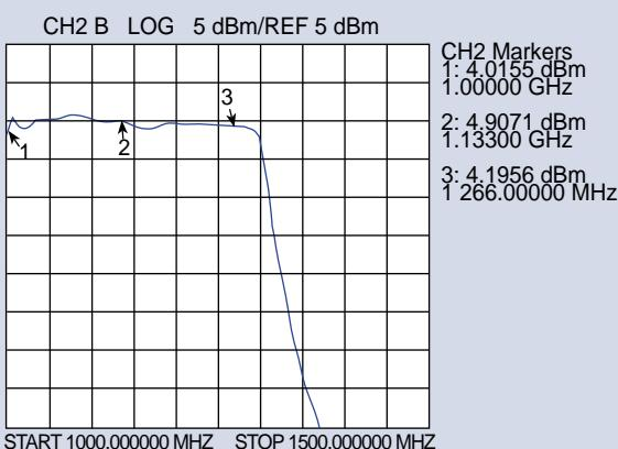
Tripler Output Power Flatness (3000-3800 MHz Output)
