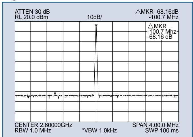
Multiplier Spectral Purity (Close Spectrum @ 25°C)
