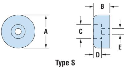
Standard color black. Standard material SBR (Styrene Butadiene Rubber), 60-70 durometer.
