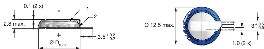
Fig. 6 - Form D2: Surface Mount Flat (single cell, keyed polarity)
