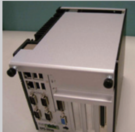
Easily Remove Top Cover by Hand
