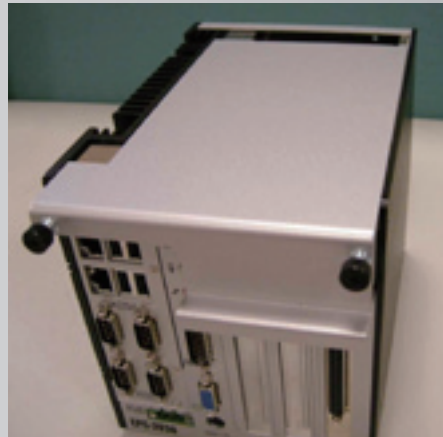
Easily Remove Top Cover by Hand
