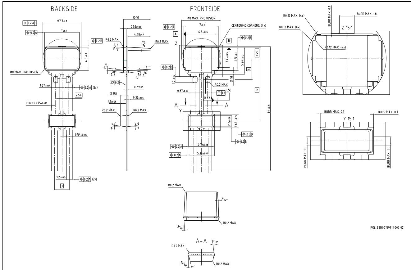
Figure 4-3 Package Outline Dimensions in mm of PG-SSOM-2-11
