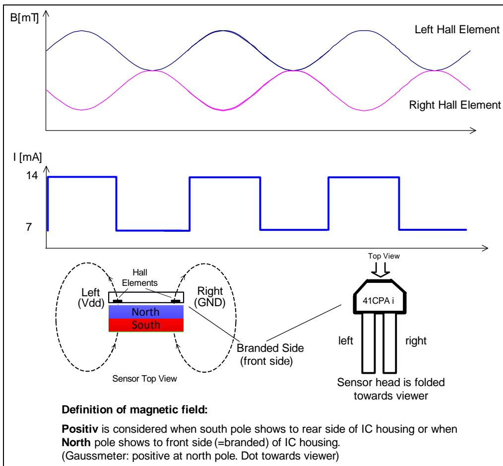
**Figure 3-2 Definition of field direction and sensor switching**
