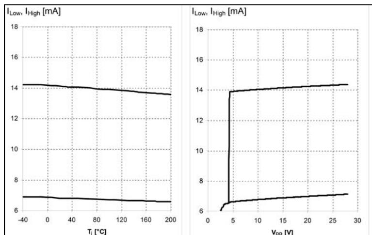
**Figure 3-5 Supply Current =*f*(*T*) (left), Supply Current =*f*(*V*<sub>DD</sub>) (right)**
