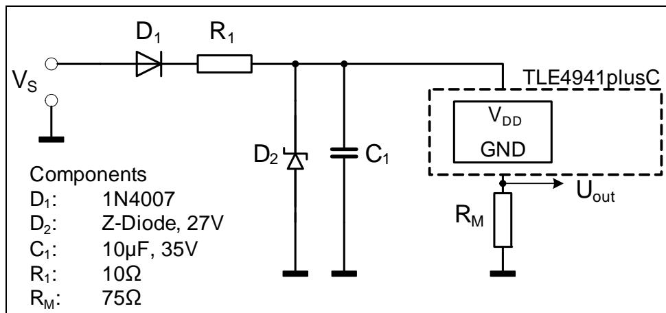
**Figure 3-4 Application Circuit**
