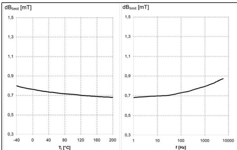
**Figure 3-7 Magnetic Threshold  $\Delta B_{\text{Limit}} = f(T)$  at  $f = 200\text{Hz}$  (left), Magnetic Threshold  $\Delta B_{\text{Limit}} = f(f)$  (right)**
