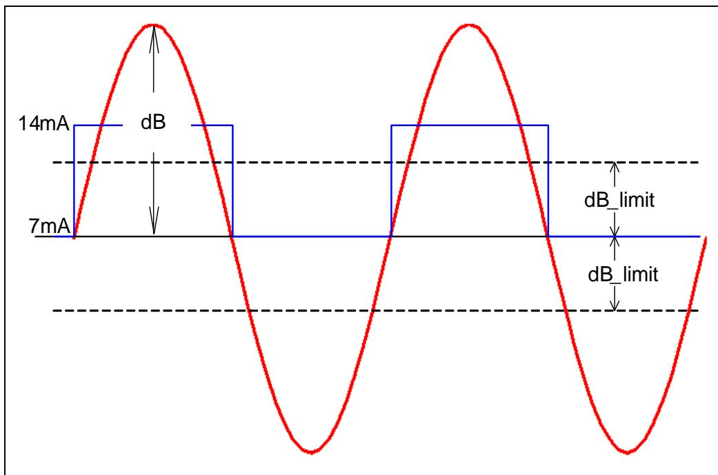
**Figure 3-1 Description of differential field  $\text{dB}$  and switching threshold  $\text{dB}_{\text{limit}}$  (calibrated mode)**
