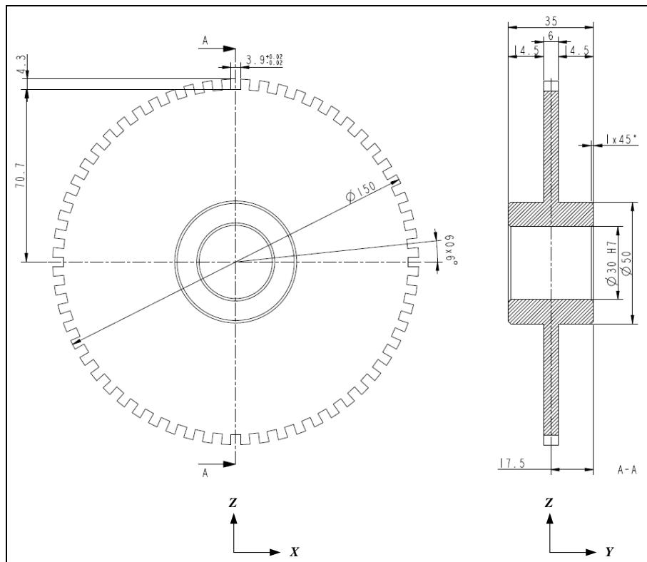
**Figure 3-9 Top view of reference target wheel**
