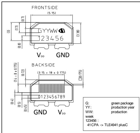
Figure 2-1 Front side and Backside Marking of PG-SSO-2-53
