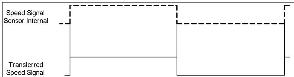
**Figure 2-3 Speed Signal (half a period =  $0.5 \times 1/f_{\text{speed}}$ )**
