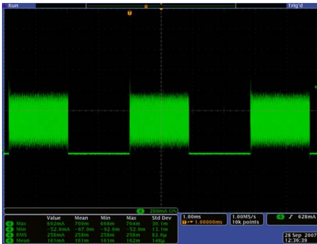
FIGURE 10. I_L AT 50% PWM DIMMING (54 LEDs, 20mA, V_{IN} = 12V , L = 8.2\mu H )
