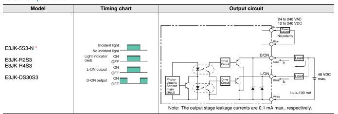
Note: Connect the brown cable to any polarity and the blue cable to the power supply because there is no polarity on the Emitter side. \* Models numbers for Through-beam Sensors (E3JK-5□□-N 2M) are for sets that include both the Emitter and Receiver.
