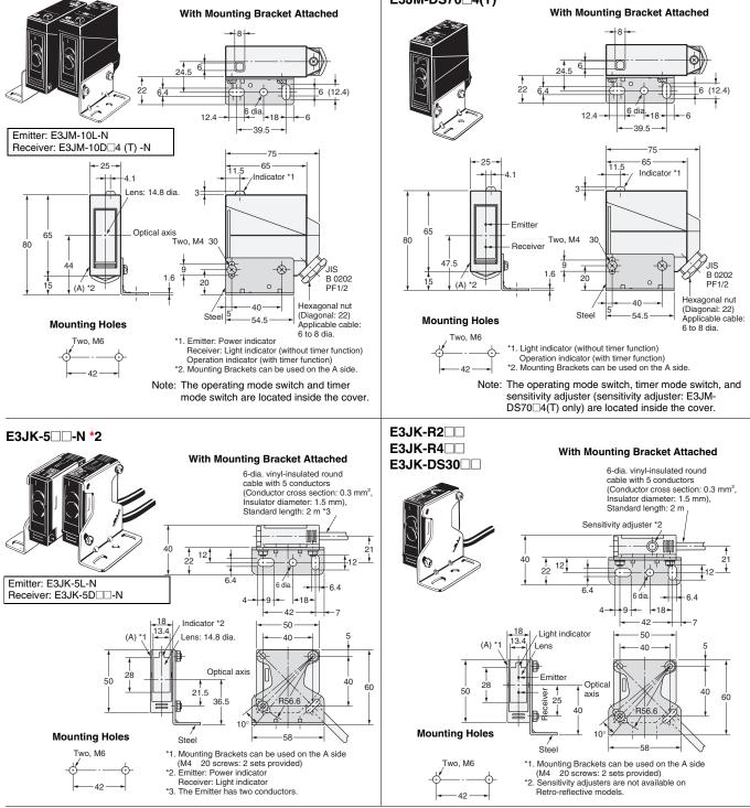
\*1. Models numbers for Through-beam Sensors (E3JM-10□4(T)-N) are for sets that include both the Emitter and Receiver.
