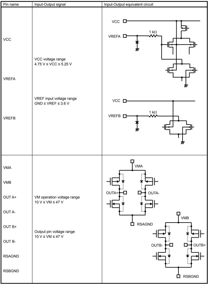
Note: The equivalent circuit diagrams may be simplified or omitted for explanatory purposes.
