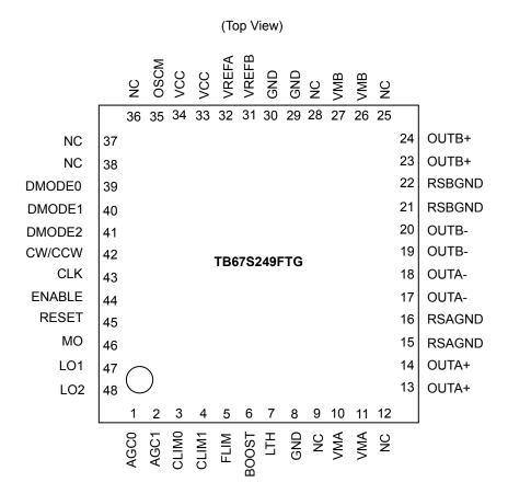
Note: Please solder the corner pad and the rear thermal pad of the QFN package, to the GND pattern of the PCB.
