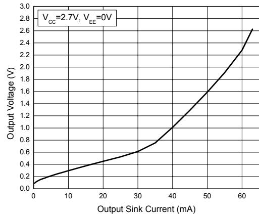
Figure 9. Output Voltage vs. Output Sink Current
