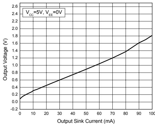
Figure 8. Output Voltage vs. Output Sink Current
