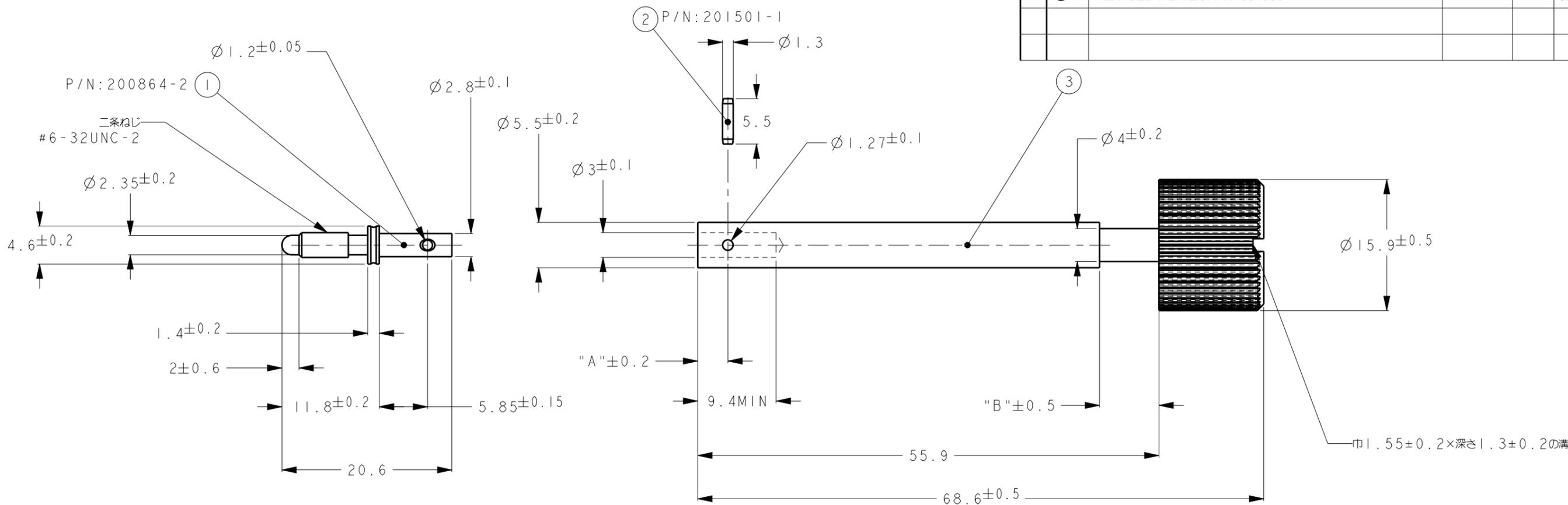
1. TO PREVENT THREAD STRIPPING, SCREW TORQUE SHOULD NOT EXCEED 12kg-cm Max
