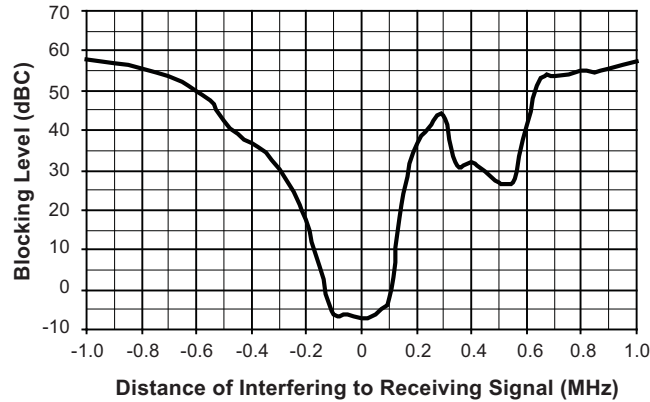
Figure 5-3. Close In 3dB Blocking Characteristic and Image Response at 433.92MHz
