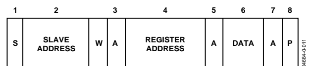
Figure 11. Single-Byte Write to a Register
