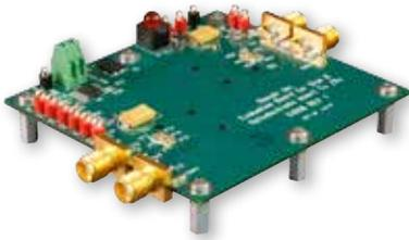
The 050-301-EVALBOARD (Size 8 evaluation board) can be used in one of three test configurations to test active size 8 opto-electronic contacts (part numbers: 050-301, 050-307, 050-308 ). The options are:
