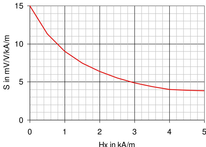
Auxiliary field strengths below  $H_x < 1.5 \text{ kA/m}$  are not recommended, as small disturbances may flip the magnetization domains. Sometimes, the magnetic conditions in the application may provide enough  $H_x$  bias field stabilization. MEAS Germany can provide advice for customer specific magnet arrangements.
