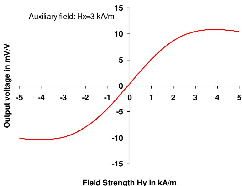
**Figure 4:** Characteristic output curve of KMY 20 S / KMY 22 S / KMZ 20 S for an auxiliary field strength of  $H_x=3 \text{ kA/m}$
