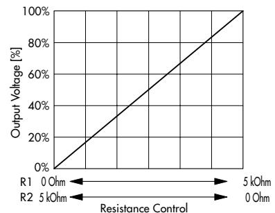
Connection for remote control voltage control
