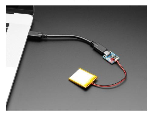
Charging is performed in three stages: first a preconditioning charge, then a constant-current fast charge and finally a constant-voltage trickle charge to keep the battery topped-up. The charge current is 100mA by default, so it will work with any size battery and USB port. If you want you can easily change it over to 500mA mode by soldering closed the jumper on the front, for when you'll only be charging batteries with 500mAh size or larger.
