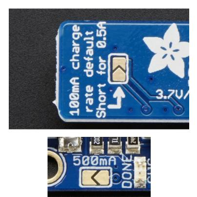
Melt some solder onto the jumper to close it and set the new charge rate
