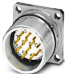
Device connector for front wall, straight, shielded: yes, for standard and SPEEDCON interlock, M23, No. of pos.: 17, type of contact: Pin, Solder-in connection, Flat gasket, 4x Ø 3.2, flange dimensions: 25 mm x 25 mm
