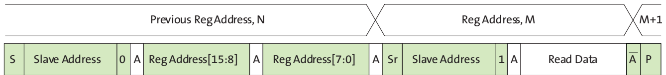
Figure 9: Single READ from Random Location
