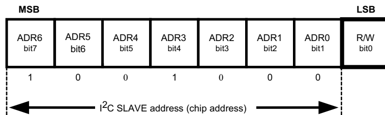
Figure 32. I²C Chip Address
