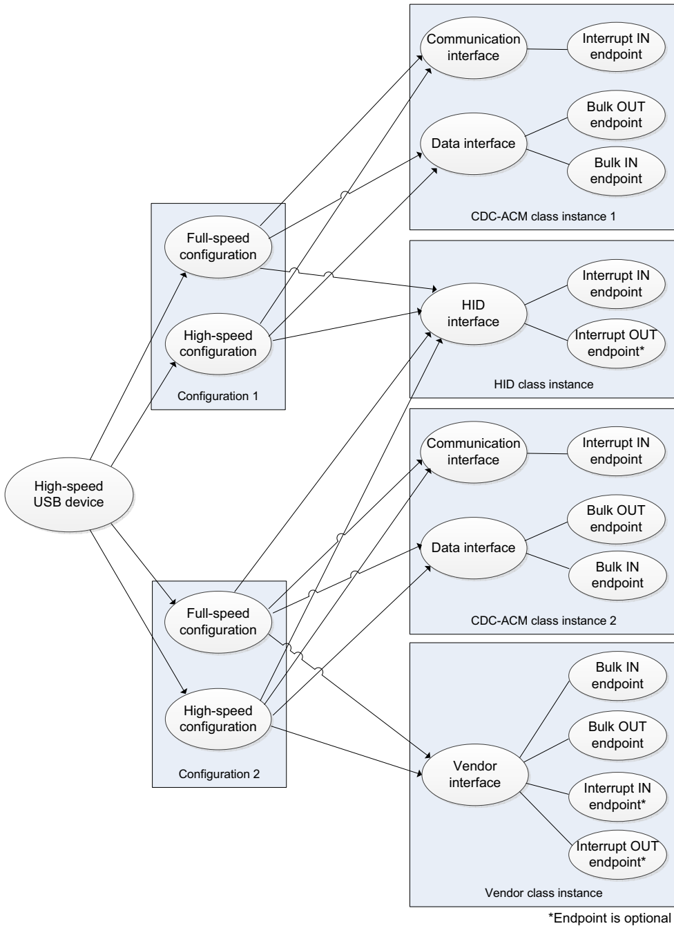
Figure 5-2 Complex Composite High-Speed USB Device Structure
