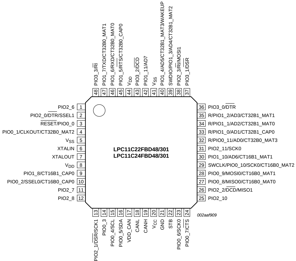
Fig 3. Pin configuration (LPC11C22/C24)
