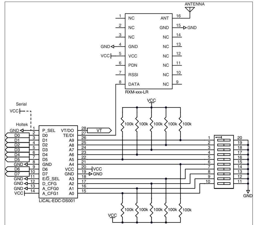
Figure 11: LR Receiver and DS Decoder Schematic
