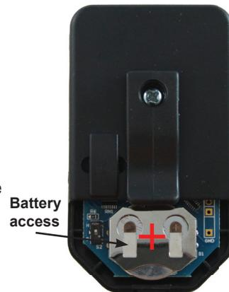
Figure 8: Battery Access
