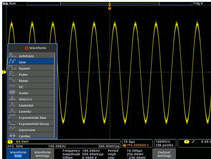
Waveform type selection in the integrated AFG.
