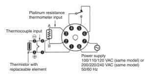
On the E52-\(\sigma\) 1D, the lead wires are thermocouple element wires, making them difficult to solder because solder will not stick to them easily. Remove the crimp terminal and polish the ends before attempting to solder them.
