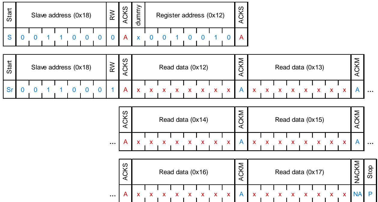
Figure 5: I 2 C multiple read
