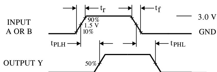
**Figure 1. Switching Waveforms**
