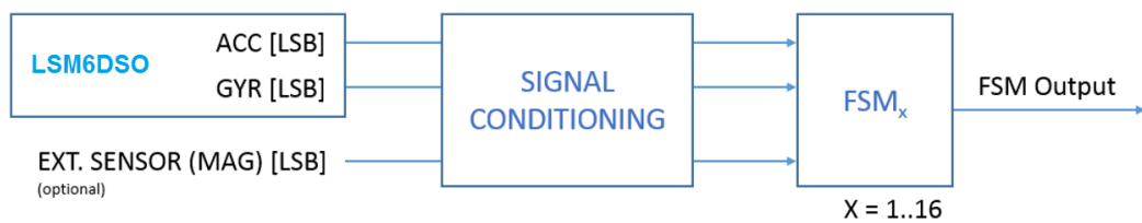
Figure 2. State machine in the LSM6DSO
