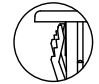
DETAIL VIEW VHP CONTURA X, XI & XII HOLE PLUGS (With wing serrations)
