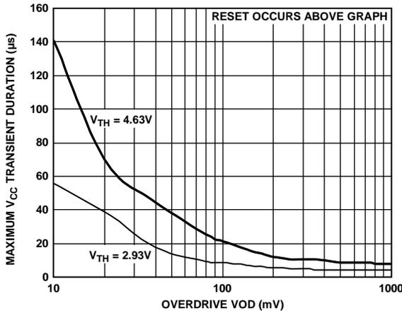
Figure 12. Maximum V<sub>CC</sub> Transient Duration vs. Reset Threshold Overdrive
