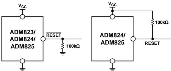
Figure 17. Ensuring Reset Valid to  $V_{CC} = 0$  V
