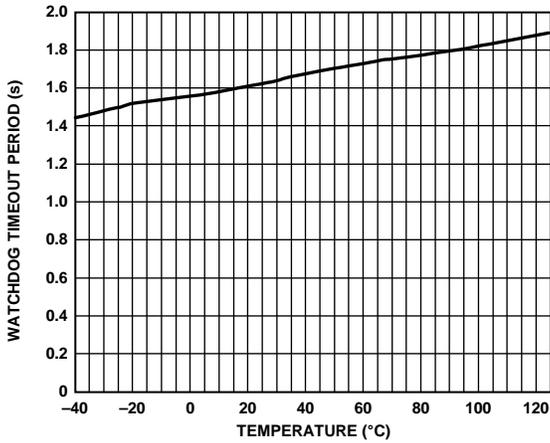
Figure 11. Watchdog Timeout Period vs. Temperature (ADM823/ADM824)
