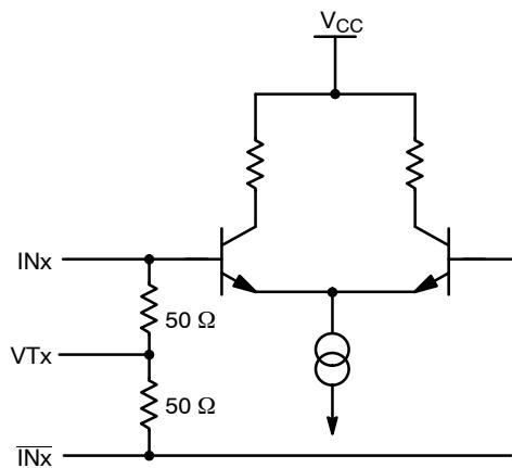
**Figure 4. Input Structure**
