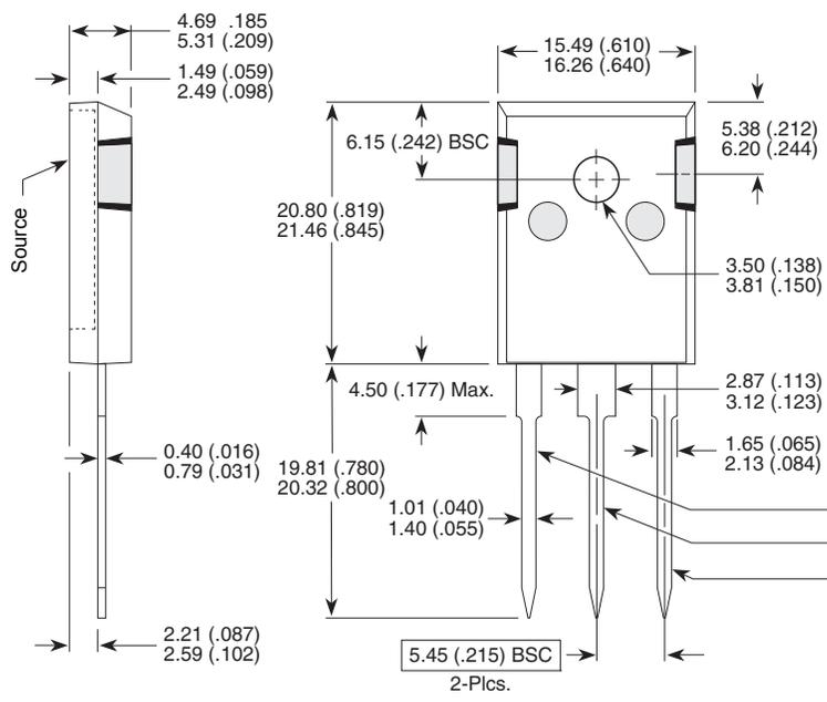
**NOTE:** These two parts comprise a symmetric pair of RF power transistors and meet the same electrical specifications. The device pin-outs are the mirror image of each other to allow ease of use as a push-pull pair.
