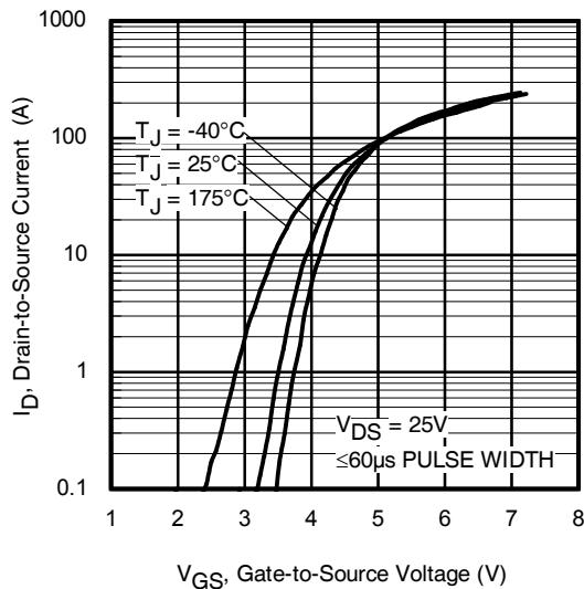
**Fig. 5.** Transfer Characteristics
