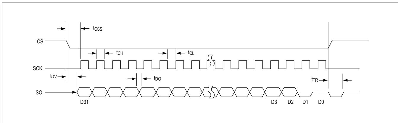
Figure 2. Serial-Interface Timing
