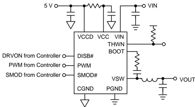
Figure 1. Application Schematic
