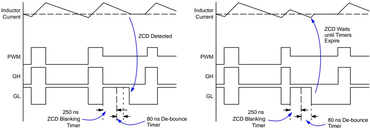
NOTES: If the Zero Current Detect circuit detects zero current after the ZCD Wait timer period, the GL is driven low by the Zero Current Detect signal.
