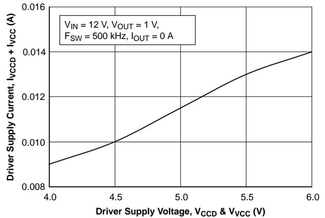
**Figure 14. Driver Supply Current vs. Driver Supply Voltage**
