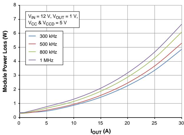
**Figure 7. Power Losses vs. Output Current, 12  $V_{IN}$**
