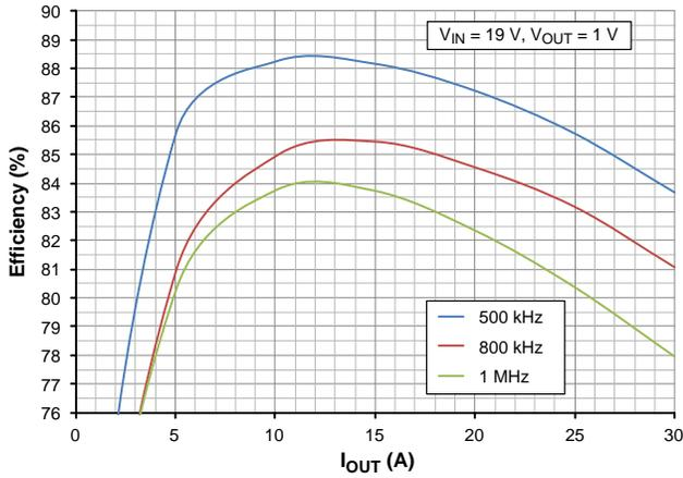
**Figure 3. Efficiency – 19 V Input, 1.0 V Output**
