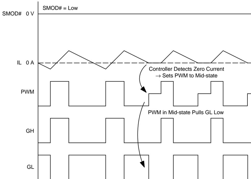
**Figure 17. Timing Diagram – 3-State PWM Controller, with ZCD**
