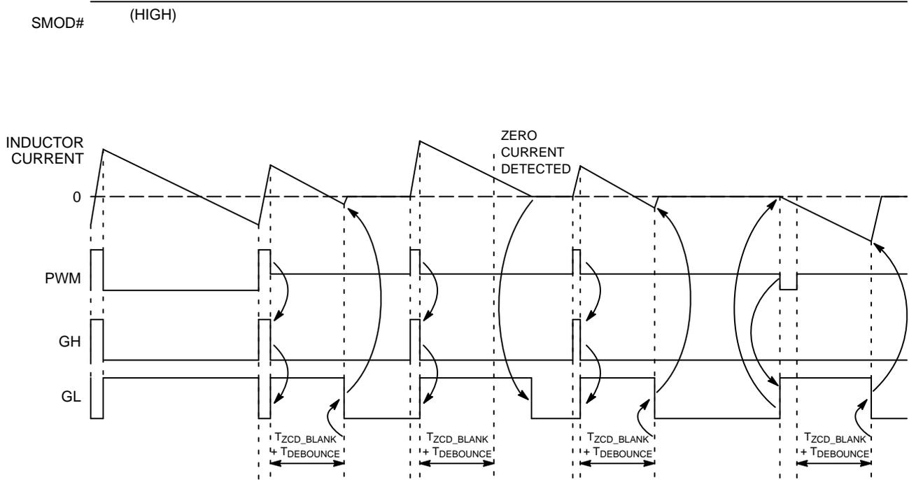
**Figure 16. Timing Diagram – 3-State PWM Controller, No ZCD**
