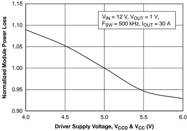
**Figure 11. Power Loss vs. Driver Supply Voltage**
