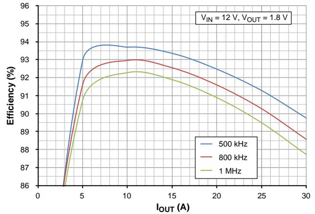
**Figure 6. Efficiency – 12 V Input, 1.8 V Output**
