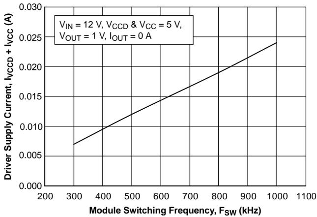
**Figure 13. Driver Supply Current vs. Switching Frequency**
