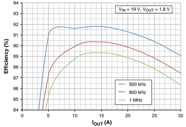
**Figure 4. Efficiency – 19 V Input, 1.8 V Output**
