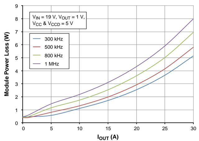
**Figure 8. Power Losses vs. Output Current, 19  $V_{IN}$**
