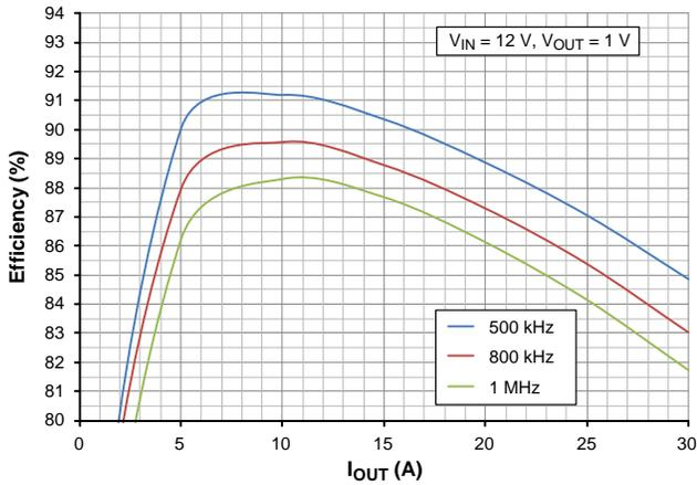
**Figure 5. Efficiency – 12 V Input, 1.0 V Output**
