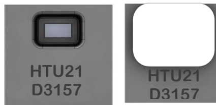
Laser marking on HTU21D(F) sensor
