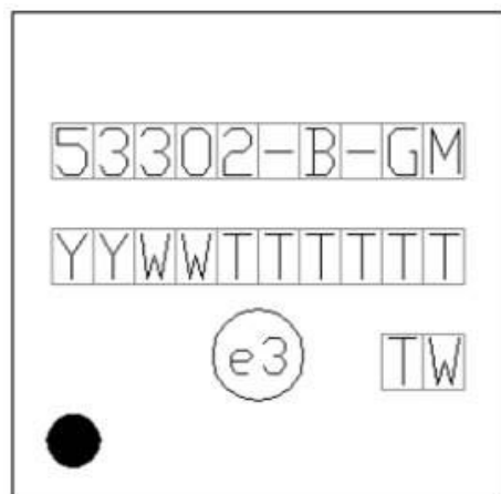
Figure 8.4. Si53302 Top Marking
