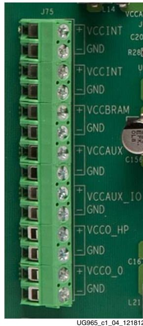
Figure 1-4: Core Power Terminal Block J75
