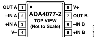
Figure 1. ADA4077-2 Pin Configuration, 8-Lead MSOP
