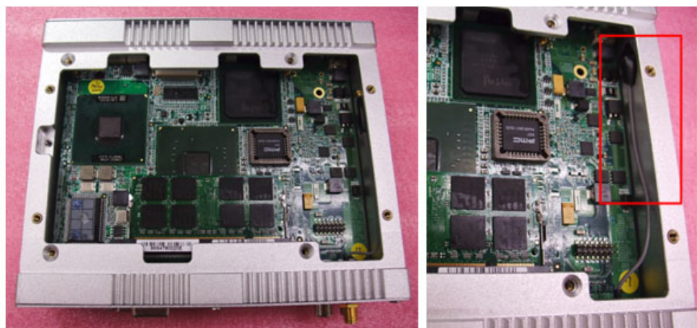
Figure 5.11 UMTS/HSDPA SMA cable internally
