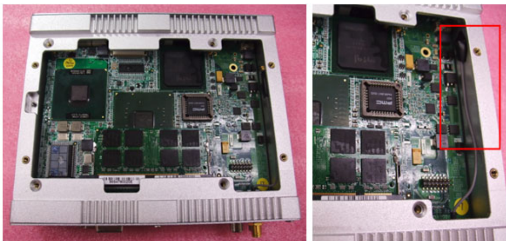
Figure 5.4 GPRS/EDGE SMA cable internally
