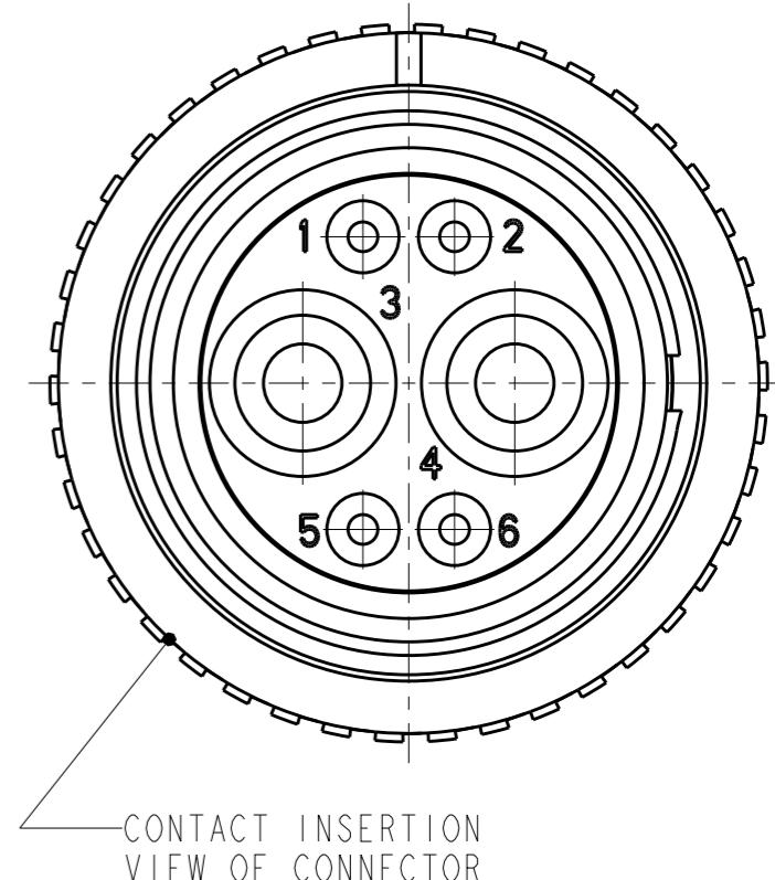
3. THIS CONNECTOR MATES WITH PART NO. HD34-18-6PX-XXXX.
