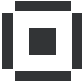
Figure 80. 82574L Silkscreen and Components Pad (Top View)
