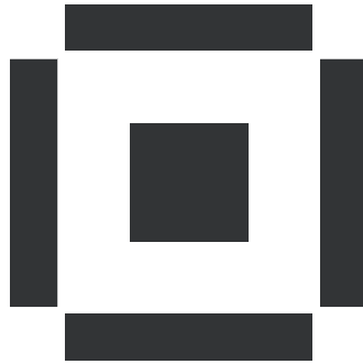
Figure 80. 82574L Silkscreen and Components Pad (Top View)
