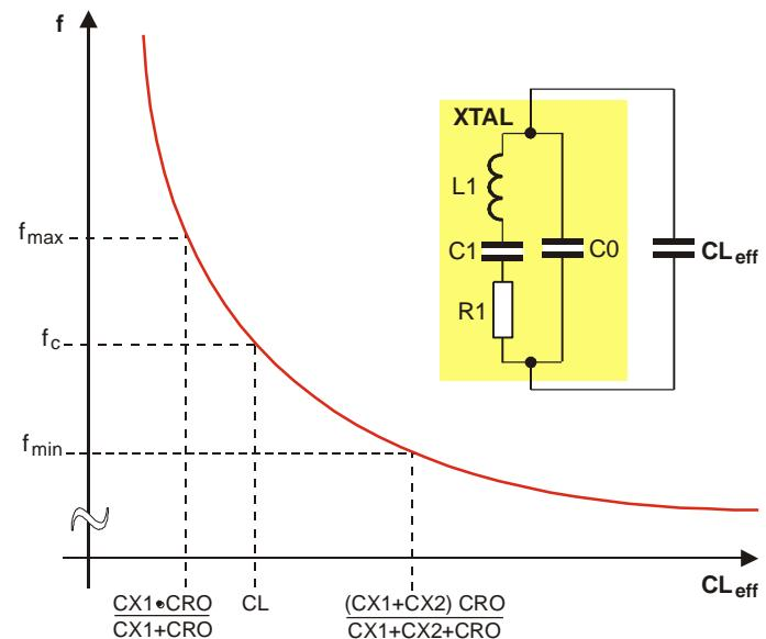
Fig. 3: Crystal pulling characteristic
