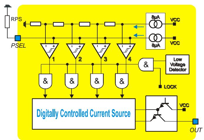
Fig. 4: Block diagram of output power control circuitry
