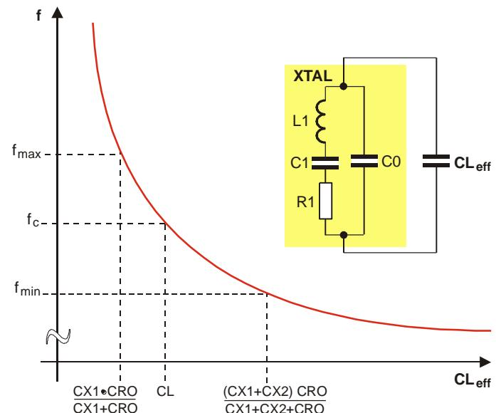
Fig. 3: Crystal pulling characteristic
