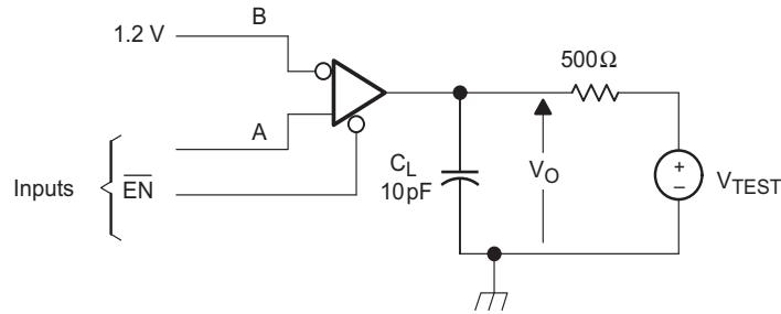
NOTE A: All input pulses are supplied by a generator having the following characteristics:  $t_r$  or  $t_f \leq 1\text{ns}$ , pulse repetition rate (PRR) = 0.5 Mpps, pulse width =  $500 \pm 10\text{ns}$ . CL includes instrumentation and fixture capacitance within 0.06m of the D.U.T.
