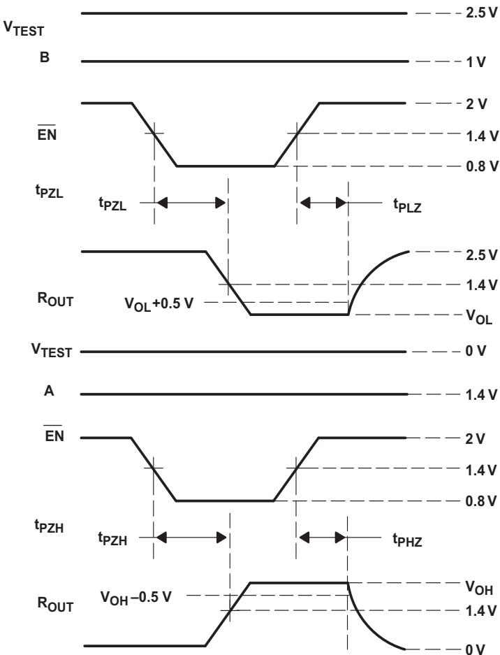
**Figure 4. Enable/Disable Time Test Circuit and Waveforms**
