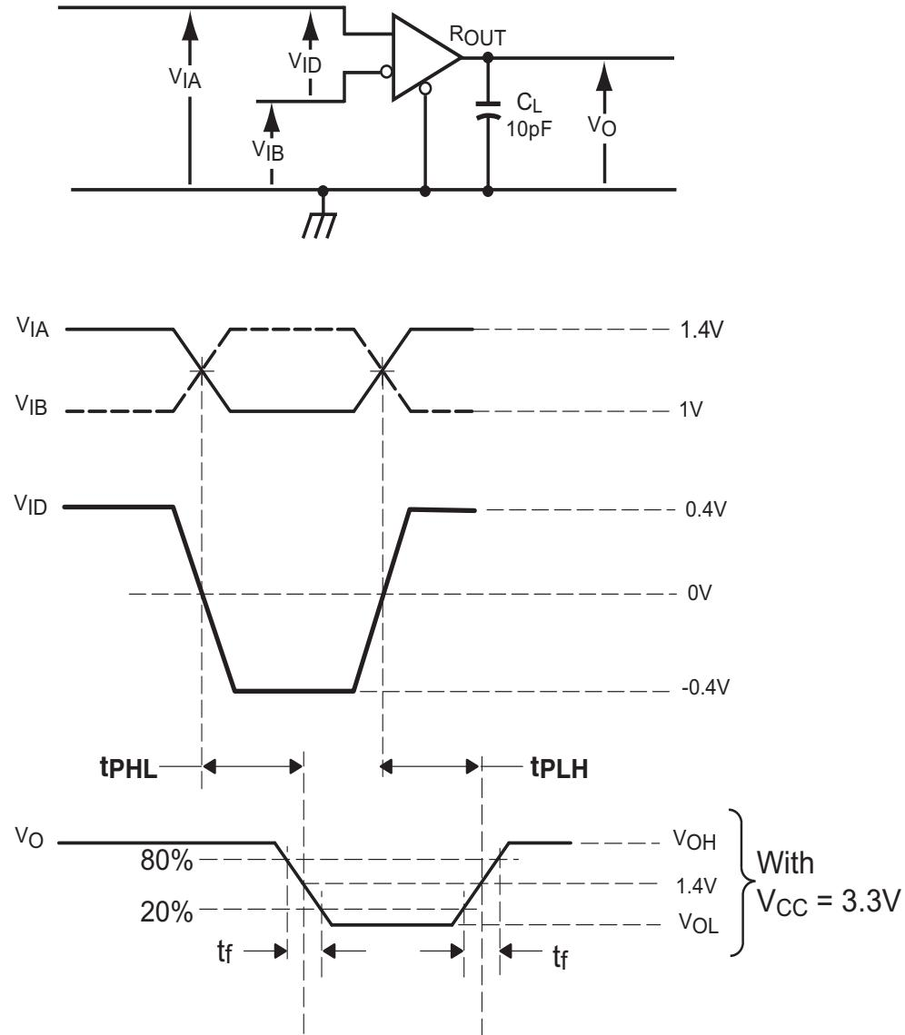
**Figure 3. Timing Test Circuit and Waveforms**
