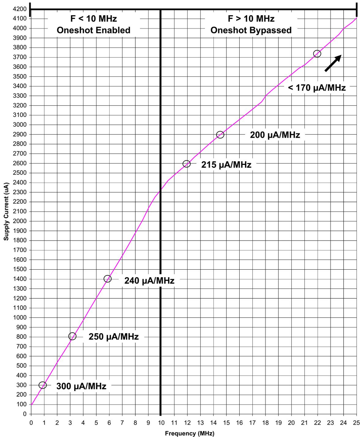
Figure 4.1. Active Mode Current (External CMOS Clock)
