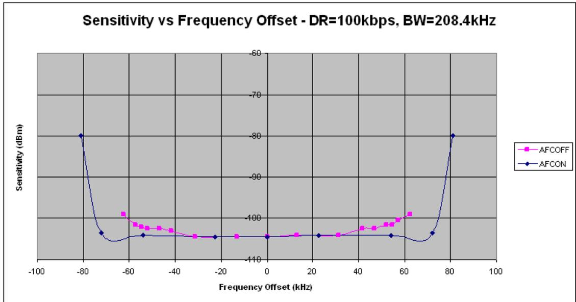
**Figure 23.5. Sensitivity at 1% PER vs. Carrier Frequency Offset**
