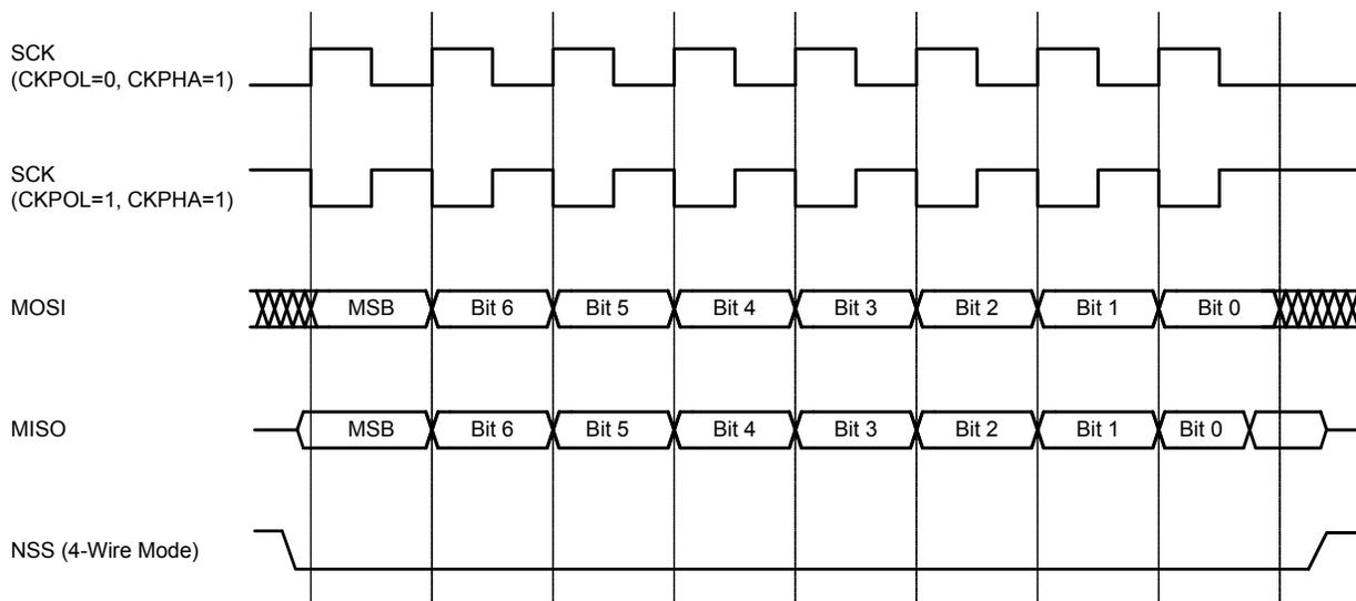
**Figure 26.7. Slave Mode Data/Clock Timing (CKPHA = 1)**
