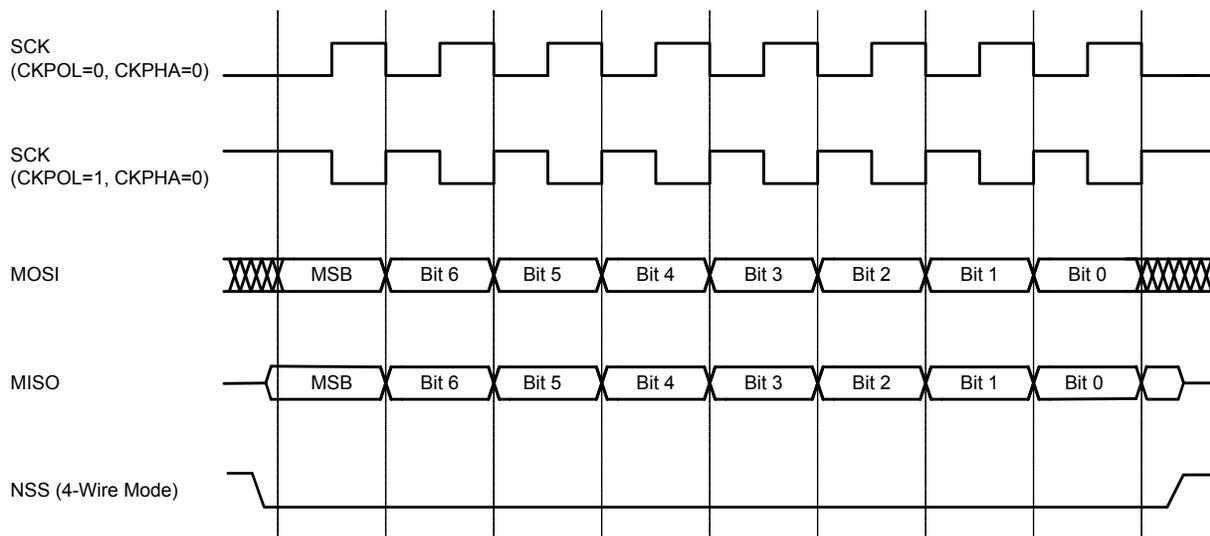
**Figure 26.6. Slave Mode Data/Clock Timing (CKPHA = 0)**
