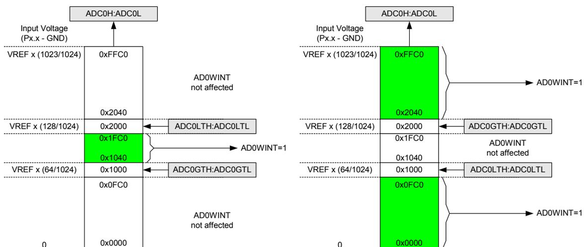
**Figure 5.6. ADC Window Compare Example: Left-Justified Single-Ended Data**
