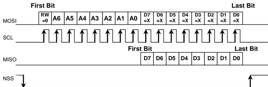
Figure 22.3. SPI Timing—READ Mode
