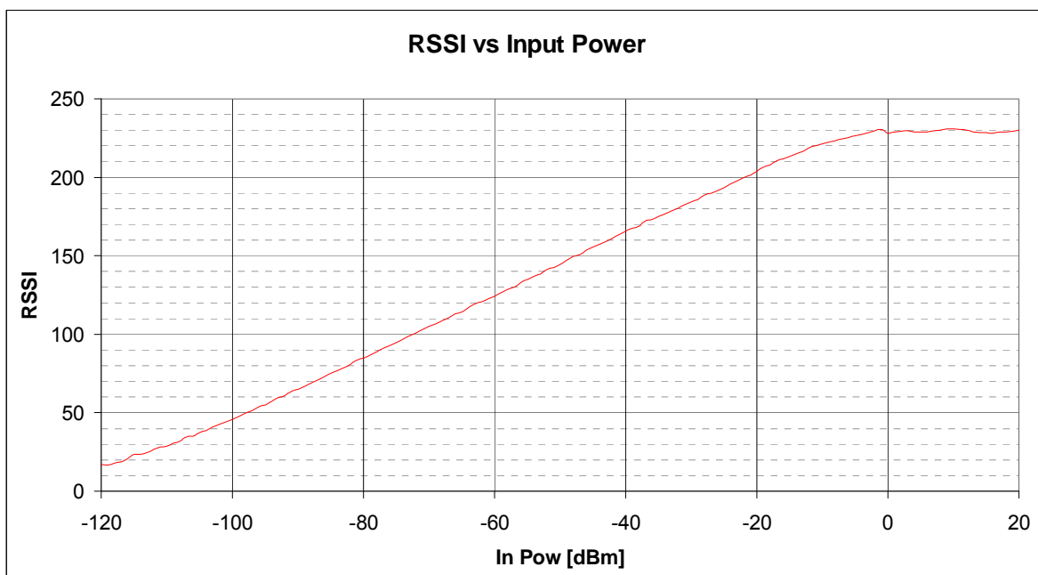
Figure 23.25. RSSI Value vs. Input Power
