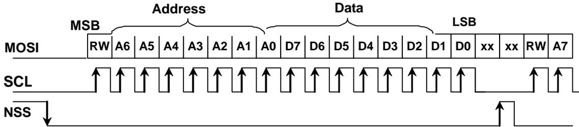
Figure 22.2. SPI Timing
