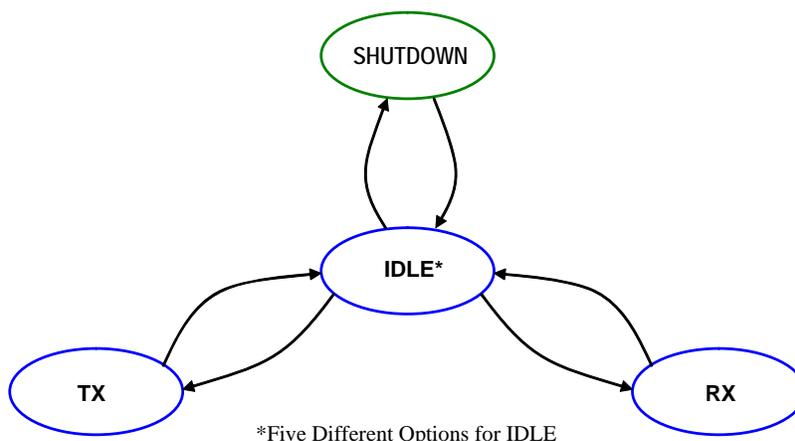
**Figure 23.1. State Machine Diagram**
