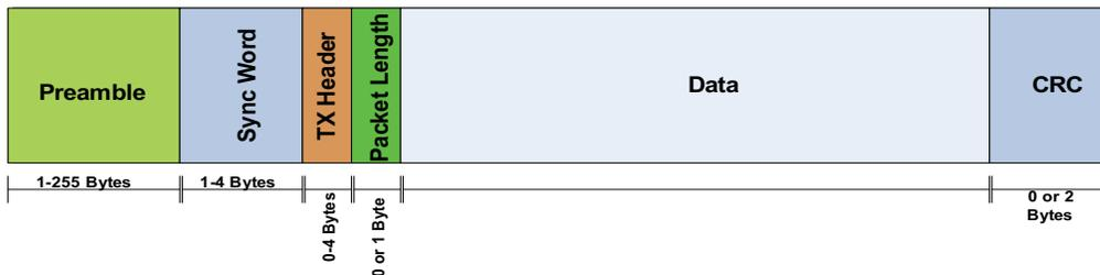
**Figure 23.12. Packet Structure**
