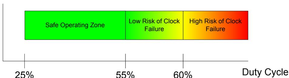
**Figure 20.2. Interpreting Oscillation Robustness (Duty Cycle) Test Results**
