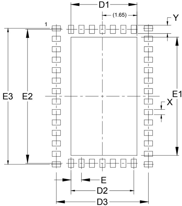
Figure 3.4. LGA-42 PCB Land Pattern Dimensions (Si1000/1/2/3/4/5-E-GM2)
