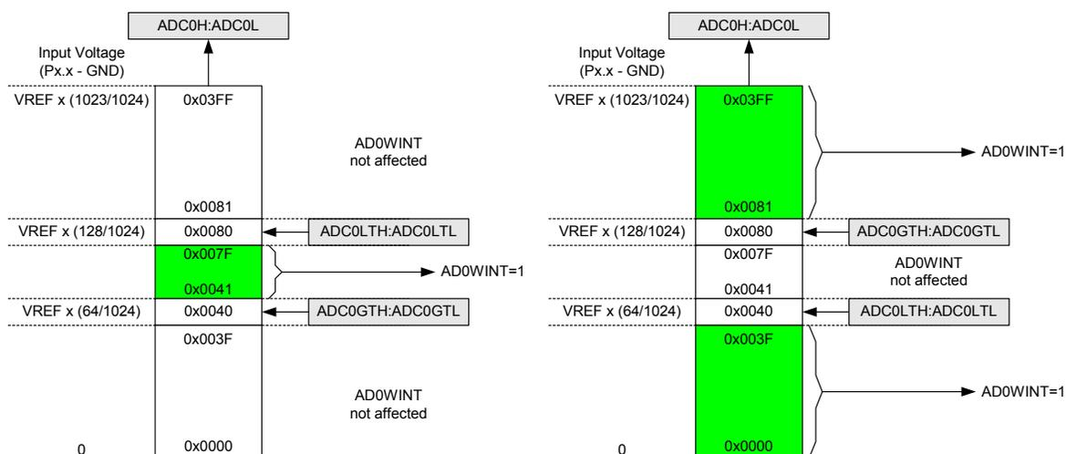
**Figure 5.5. ADC Window Compare Example: Right-Justified Single-Ended Data**
